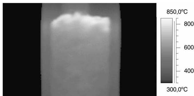
Fig. 3. Thermographic picture of the Rh1 catalyst during the autothermal tests of methane partial oxidation (residence time = 11.5 ms, reaction gas mixture \text{CH}_4/\text{O}_2/\text{He} = 2/1/4 (v/v)).
